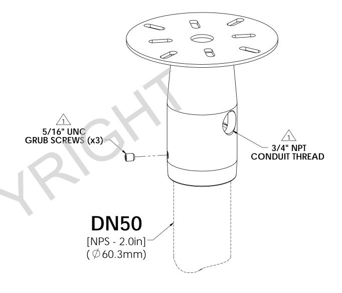
PART NUMBER = LMK6101-50-HG WEIGHT = 2.0 kg [4.4 lb] FINISH = HOT DIPPED GALVANIZED
